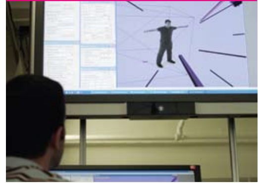
Real-time on-screen rendering of comprehensive 3D data, including 3D mesh and texture information.
